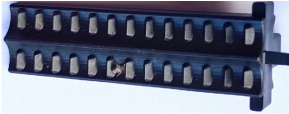
Figure 7. The new shape wedge with supports added
