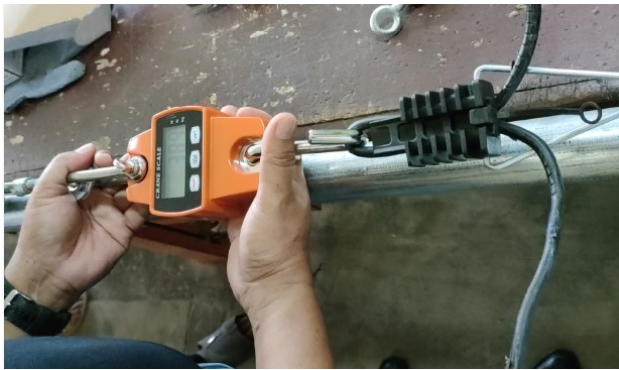
Figure 2. Tensile strength simulation test
