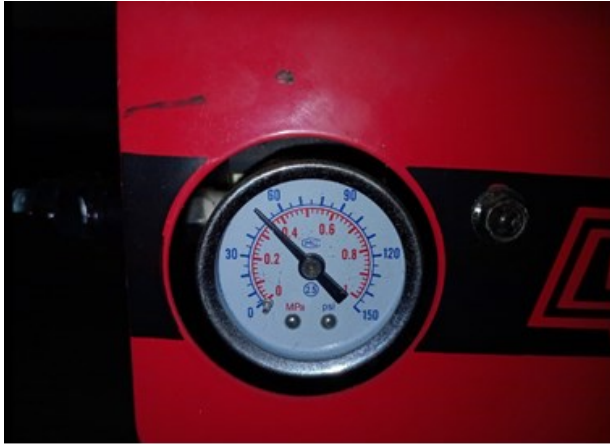
Figure 2. Pressure setup in plasma cutting machine
