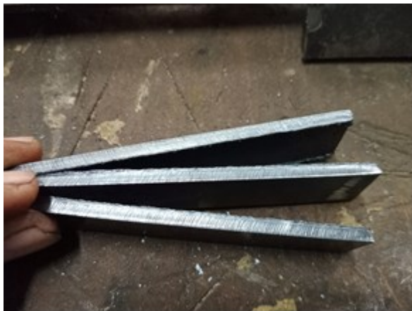
Figure 7. Cutting result with air pressure 50 psi
