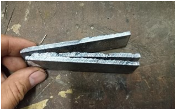
Figure 6. Cutting result with air pressure 90 psi
