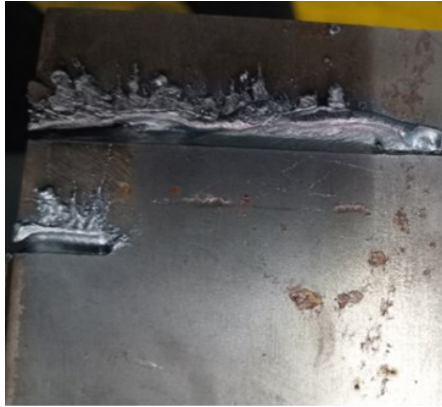
Figure 5. Cutting result with air pressure 20 psi
