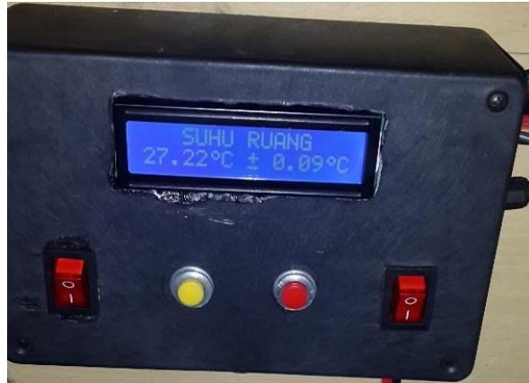
Fig. 5. Thermometer calibration LCD device display
