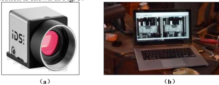
Fig. 3. Image data acquisition equipment: (a) Industrial Camera (Model: UI 3370 CP) and (b) Image data acquisition application
