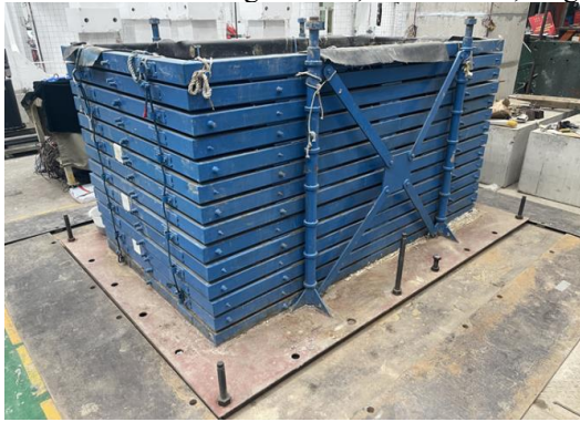
Fig. 1. Laminar shear box and shaker table top view
