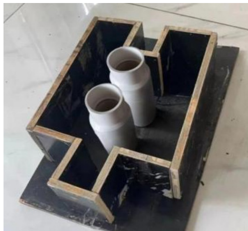
Fig. 5. Picture of PVC shrink pipe placement
