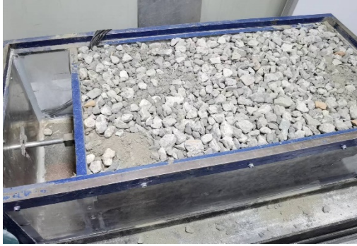
Fig. 2. Steel grid pull-out test
