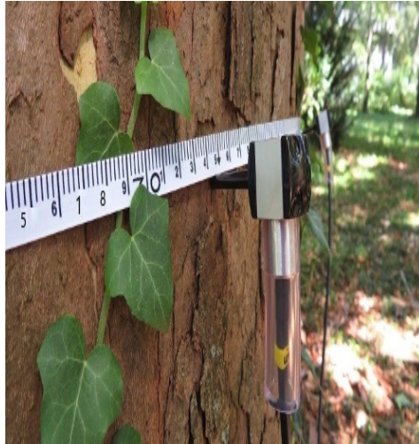
Fig. 1. Data acquisition of the interior of wood by NDT techniques
