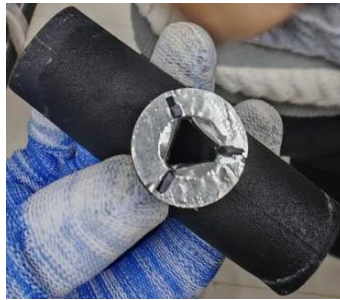
Fig. 3. Breakage Of aluminum foil membrane
