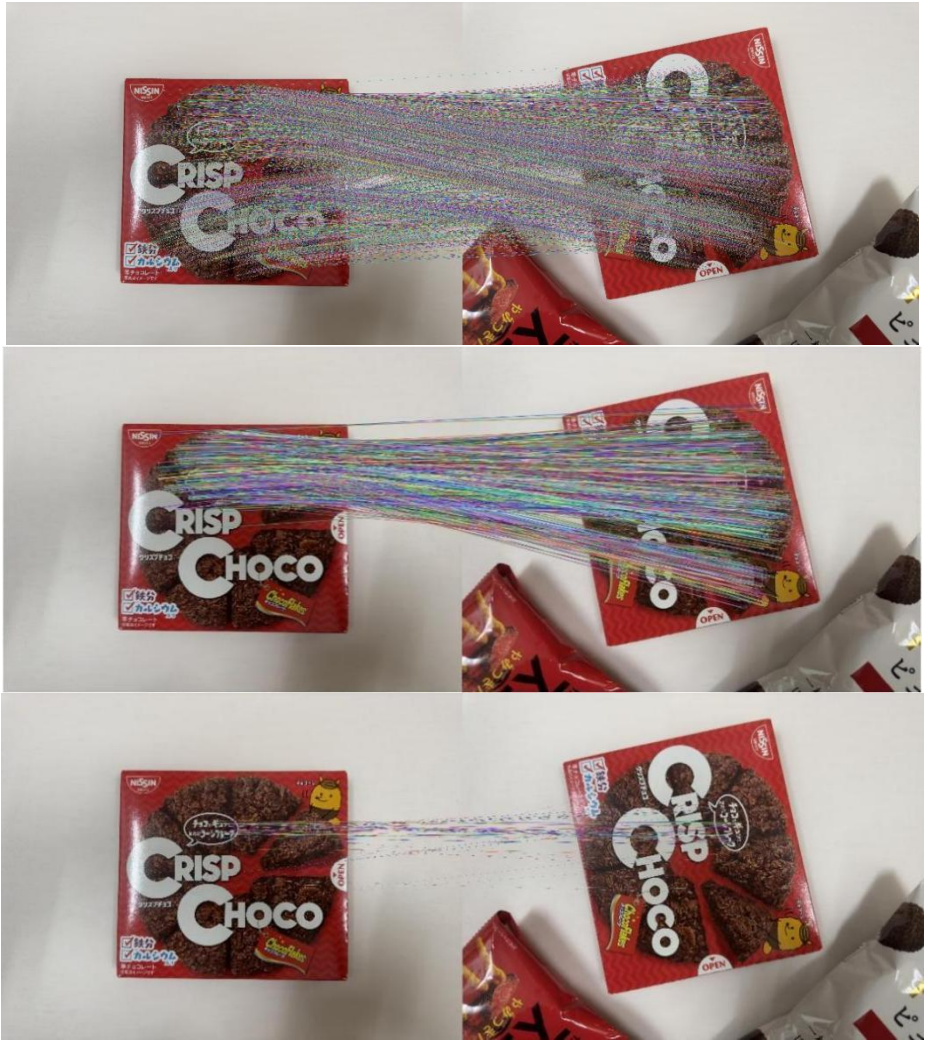
Fig. 3. Comparison of matching results of different algorithms under rotation. From top to bottom are: results of SIFT, SURF, and ORB
