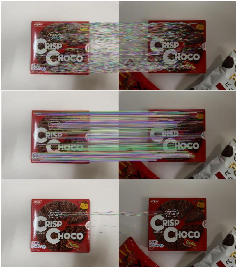
Fig. 5. Comparison of matching results of different algorithms under different light intensity. From top to bottom are: results of SIFT, SURF, and ORB
