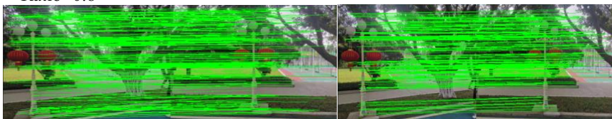
Fig. 2. Showing matching points with SIFT KAZE ORB FAST from top to bottom, left to right. (Ratio=0.6)
