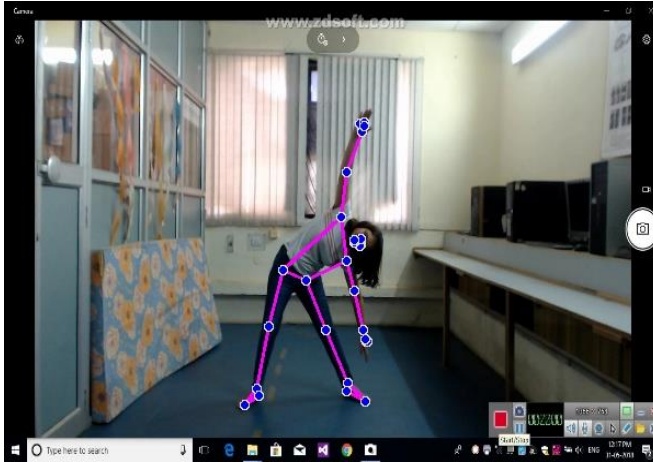
Fig. 2. Extraction of Keypoints of body parts using Mediapipe for Trikonasana video
