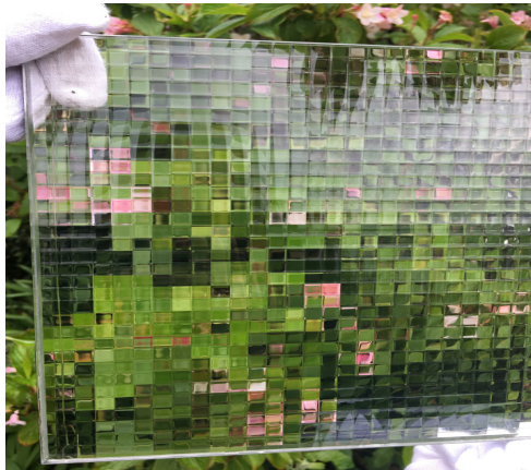
Fig. 2. Different orientations of the glass surface cause the image to be deflected as it passes through.
