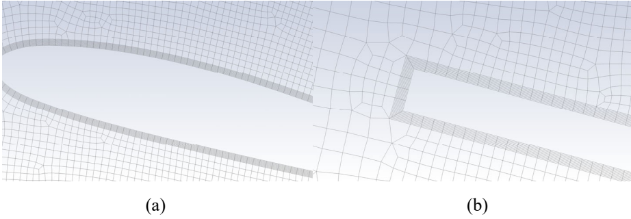
Fig. 3. Mesh division of the main wing and the tail. (a) Main wing; (b) Tail (Photo/Picture credit : Original)
