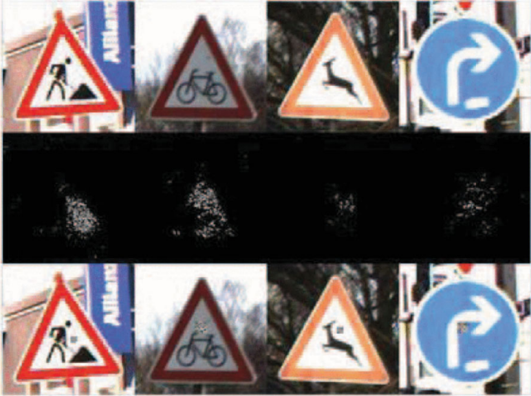
Fig. 2. Physical patch attacks against QR code-based traffic sign recognition [1].
