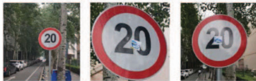
Fig. 1. Adversarial attacks schematic diagram on actual road signs [1].
