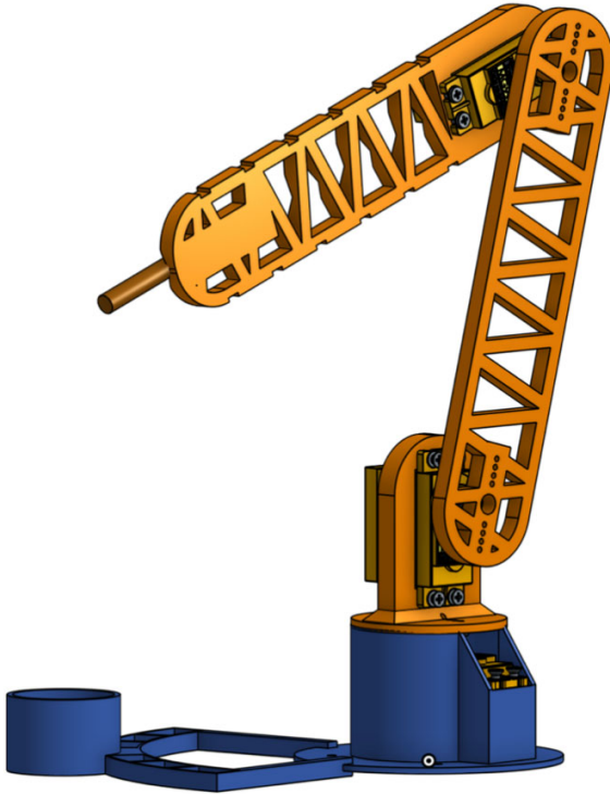
Fig. 1. A 3-Dimension Model of the 3-DOF Manipulator (Photo credited: Original)
