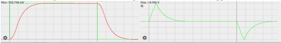
Fig. 8. The simulation results of the voltage input-angle output, and speed output (Photo credited: Original)
