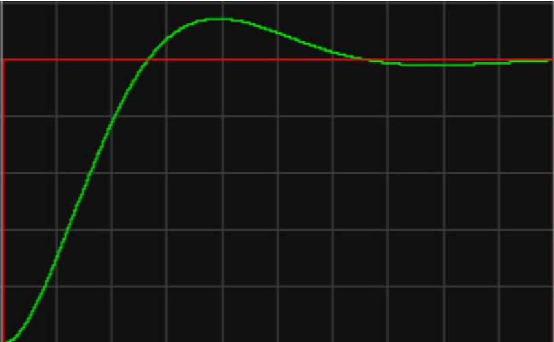
Fig. 9. Simulation result diagram under P control (Photo credited: Original)
