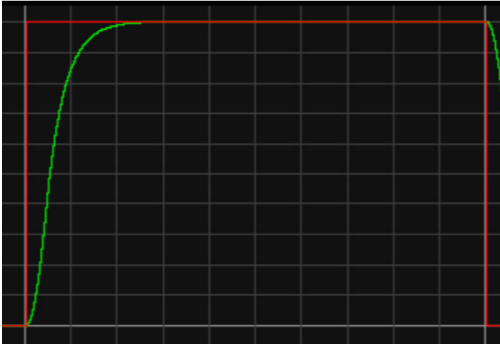
Fig. 11. Simulation result diagram under PID control (Photo credited: Original)
