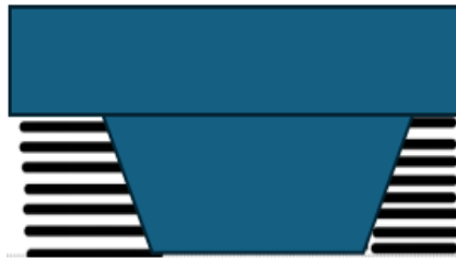
Fig. 2. FDM process principle and support (Photo/Picture credit: Original).
