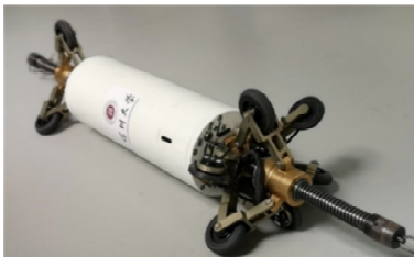
(a) Pipeline robots
