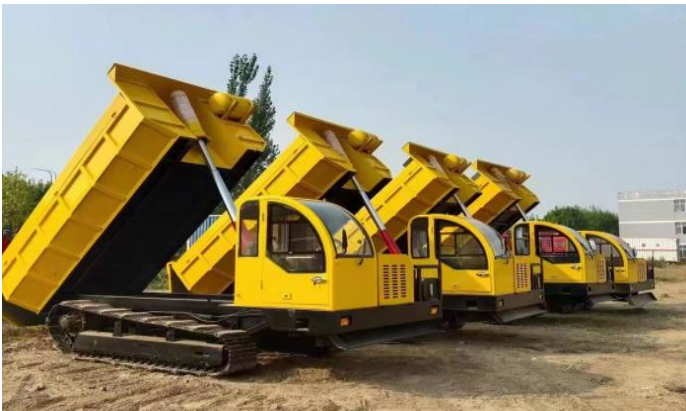
Fig. 3. Dumping Operation of Crawler Dump Truck.
