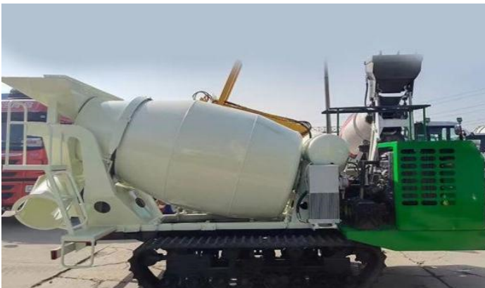
Fig. 4. Transportation of Concrete by Crawler Tanker.
