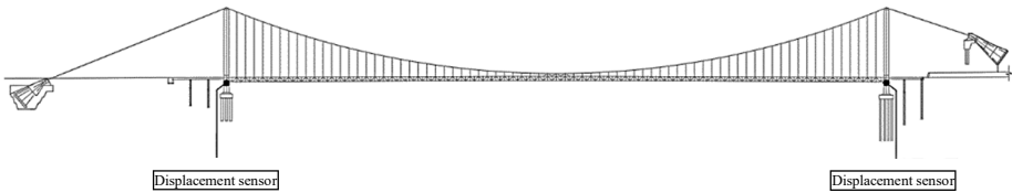
Fig. 8. Placement of tower support displacement monitoring points
