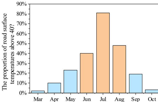
Fig. 5. Monthly Percentage of Dates with Road Surface Temperature Above 40°C
