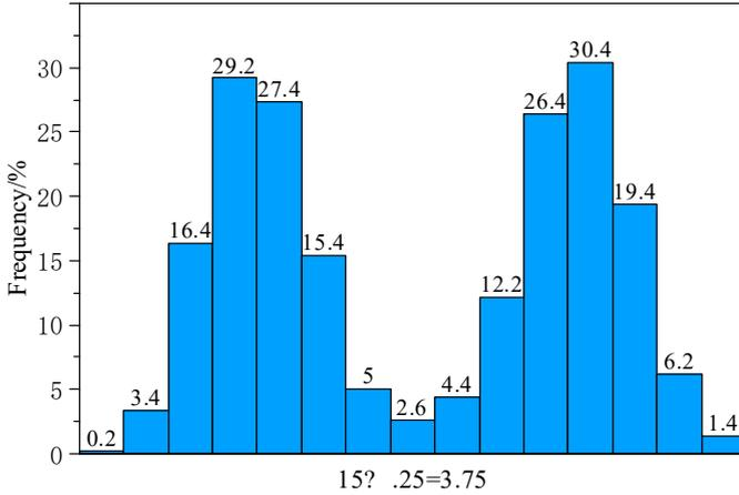
**Fig. 3.** Lateral Distribution Frequency Curve of Wheel Tracks (Single Lane Unidirectional Travel)
