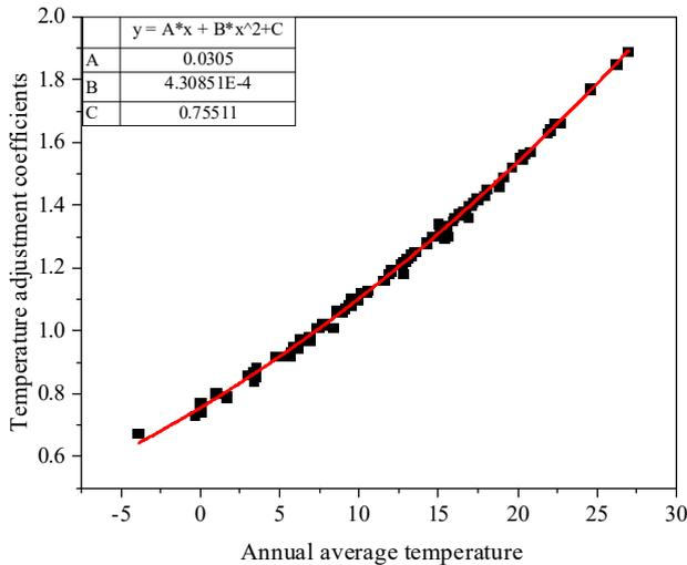
Fig. 2. Correction of Temperature Adjustment Coefficients
