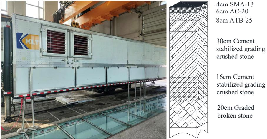
Fig. 4. ARA Full Environmental Accelerated Loading Equipment
