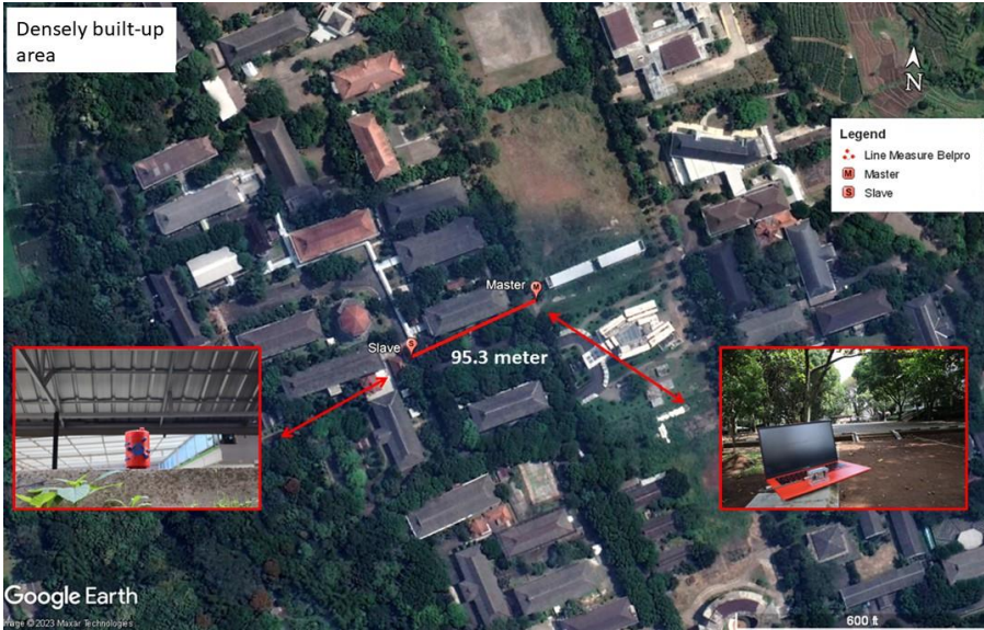
Fig 8. The connectivity range test revealed that the maximum connection distance achievable between the main unit and the node sensor is 95.5 meters.
