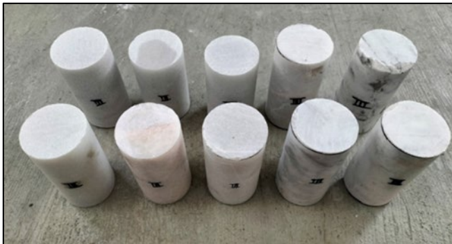
Fig. 2. The grade III cored samples of tropically weathered limestone.
