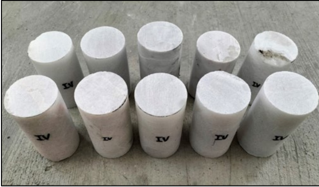
Fig. 3. The grade IV cored samples of tropically weathered limestone.
