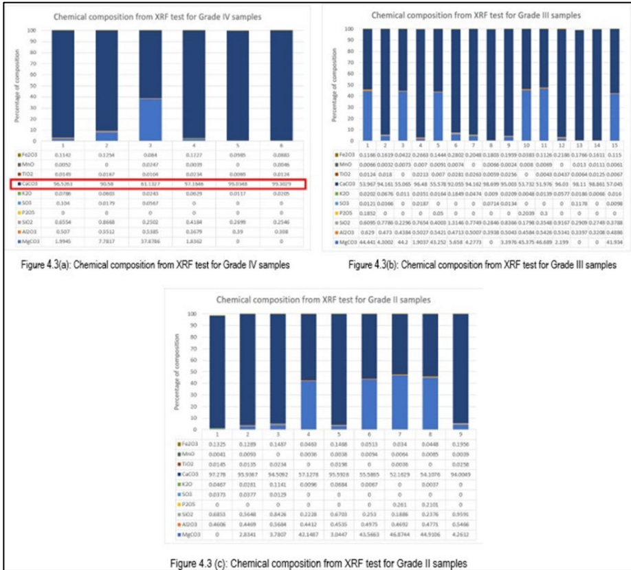
Fig. 8. Chemical composition from XRF test of the overall samples.
