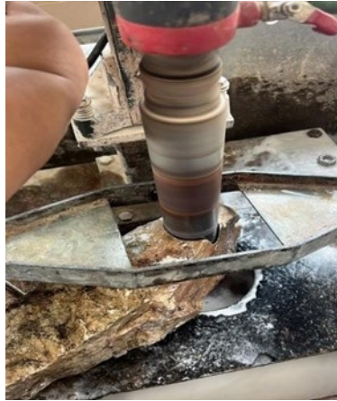
Fig. 3. Coring of limestone sample.
