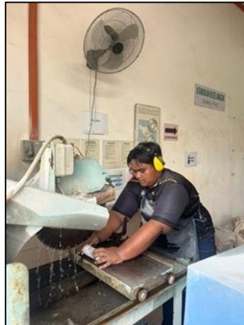
Fig. 4. Process of cutting cored limestone sample.
