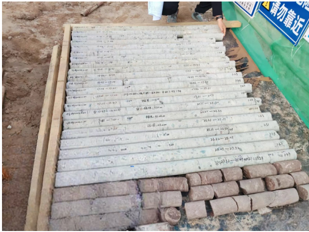
Fig. 5. Schematic diagram of concrete core samples drilled from pile foundation
