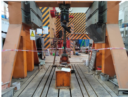
Fig. 4. PME-50A fatigue testing machine
