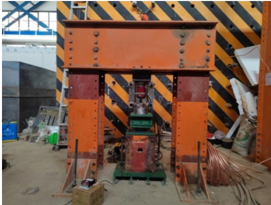
Fig. 3. Physical diagram of shear test loading
