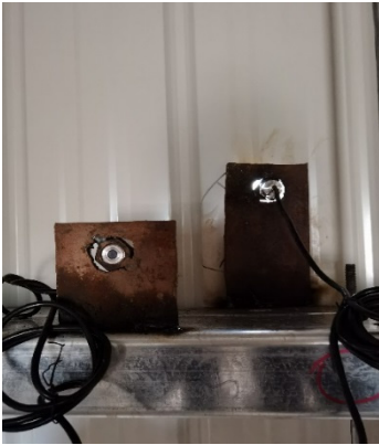
(a) Air pressure sensor
