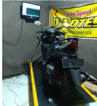
Fig 2. Engine performance testing using a dynamometer
