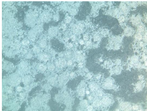
Fig 6 Microstructure of the cellular structure of the grains and sintered pore wall at 1100°C.
