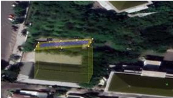
Fig 4. Side view of the solar panel placement design with an azimuth of 140^\circ and a tilt of 10^\circ .
