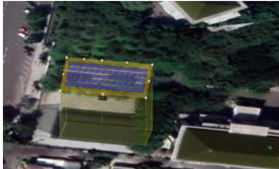
Fig 3. Side view of the solar panel placement design with an azimuth of 20^\circ and a tilt of 30^\circ .
