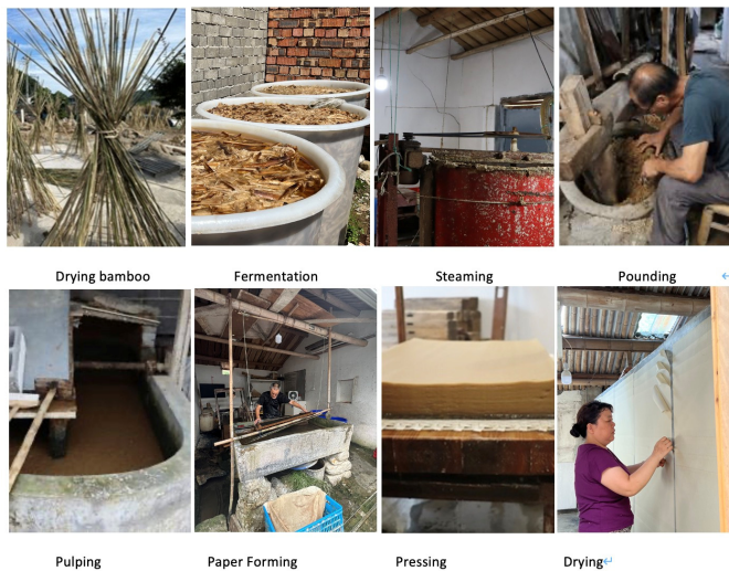
Fig. 1. The main process of traditional bamboo papermaking technique
