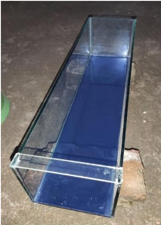
Fig. 2. Glass made open channel drain
