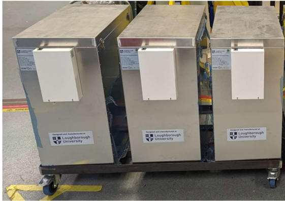
Figure 3 Photograph of three fully assembled PCM modules prepared for installation in test houses.
