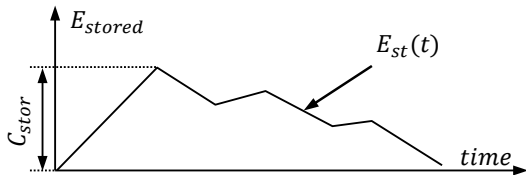
Figure 3 Calculated energy amount stored in the energy storage for each charge and discharge step during a peak period.
