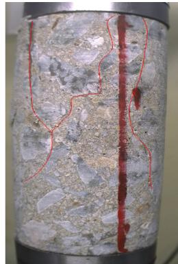
Fig. 5. Macroscopic fracture characteristics of concrete sample
