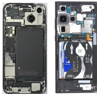
Fig. 1. Comparison of the internal structure of the Apple 15 (left) and the Samsung s23Ultra (right) (image from author's photo)
