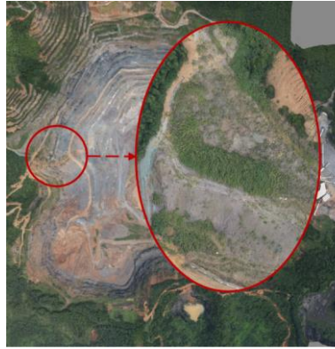
Fig. 3. the distribution of potential fractured zones in the mountainous area of the mining site
