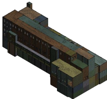
Fig. 2. The finite element model of the factory building
