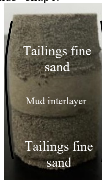
Fig. 6. Deformation of tail fine sand containing 2cm thick mud interlayer
