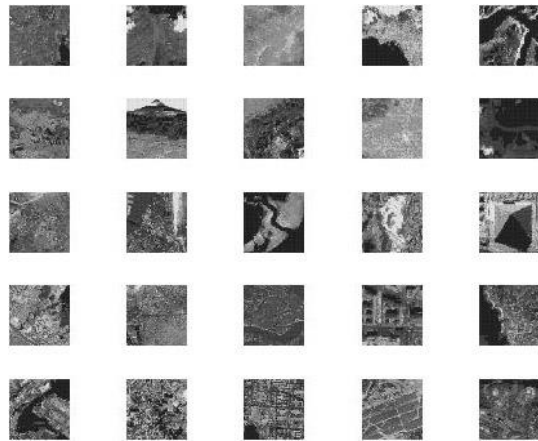
Fig. 5. Image reconstruction using block size of 4 by 4 and codebook size of 100.
