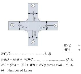
The number of lanes used for calculation purposes is determined from the average approach widths of minor roads and major roads as follows. Determine the number of lanes based on the average approach widths of minor and major roads from Figure B-1:2 below, and enter the results in Columns 9 and 10.
