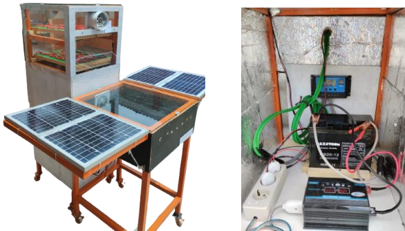
Fig. 1. Chili dryer with greenhouse effect system based on solar panel.
