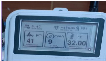
Fig. 8. Measurement result on display
