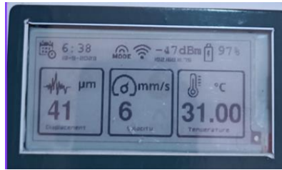
Fig. 10. Screen display in wireless sensor mode
