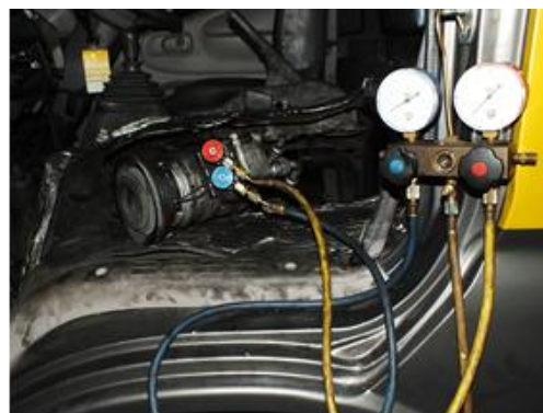
Figure 2. Draft of a Car Air Conditioning Vacuum
