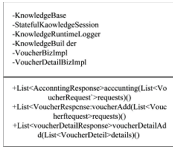
Fig. 4. Batch data receiving class diagram
