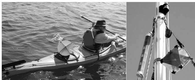
Fig. 1. The installation of radar reflector on canoe and mast of ship.
