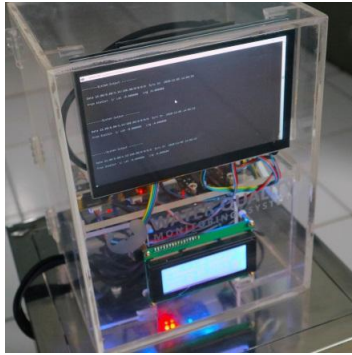
Fig. 7. Implementation of node station.
