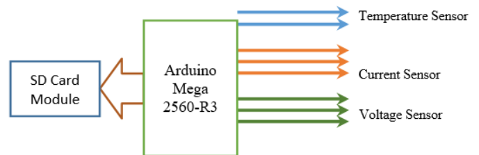
Fig. 2. Diagram block of monitoring system using Arduino mega.
