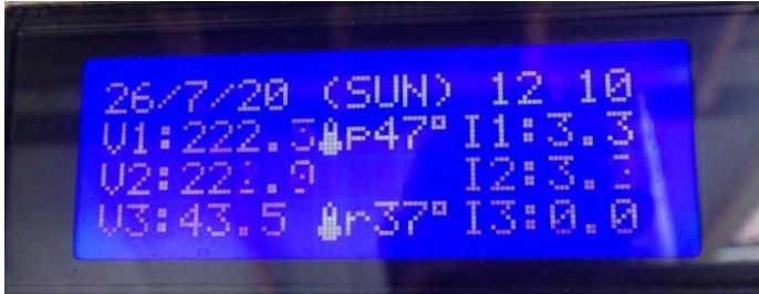
Fig. 10. LCD for displaying the acquired data in real time.
